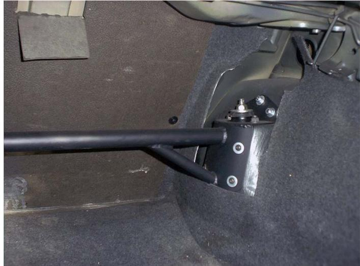
The bar can only fit one way, meaning, that the left-hand shock tower has a different shape than the right shock tower. On E30 chassis the left-hand tower, which is the driver side, appears to have less curvature than the right and also has two (2) bent corners at the top of the side skirt, also the right hand appears to have more curvature and appears to be more rounded.
